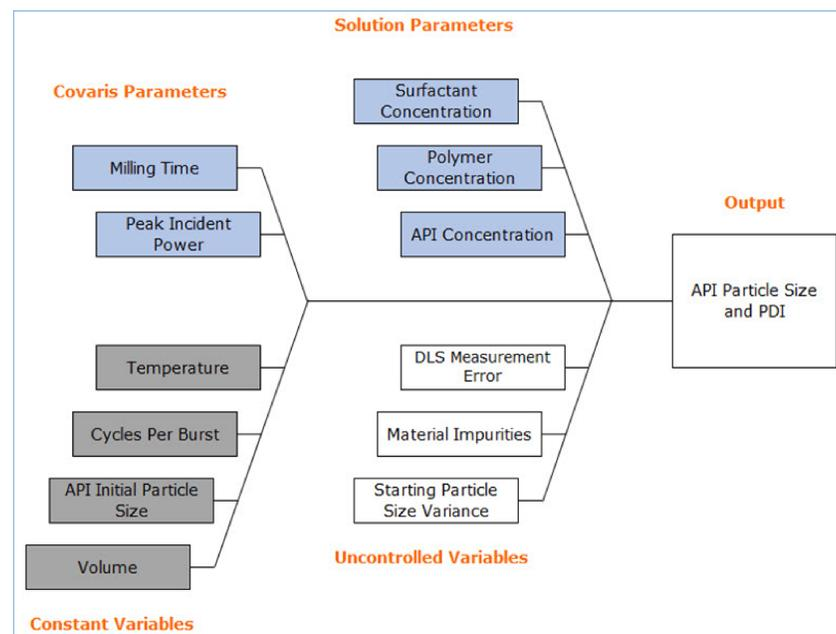
Figure 2: Parameters selected in the DOE experiment are highlighted blue. Parameters which were either controlled or showed little effect on output are in gray.
